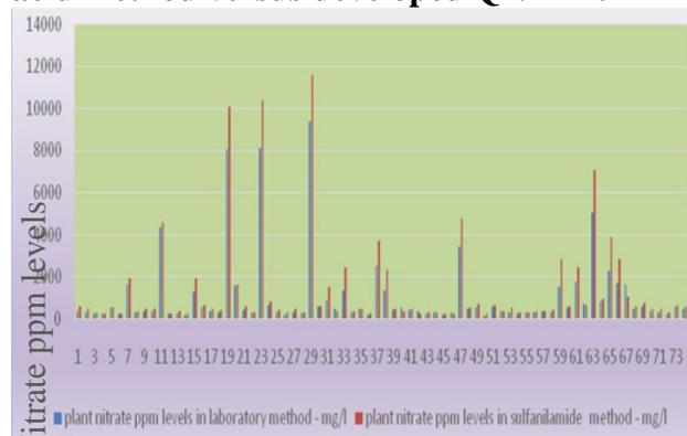
Figure 1: Comparison between standard salicylic acid methods versus developed QNT Kit (sulphanilamide method)
